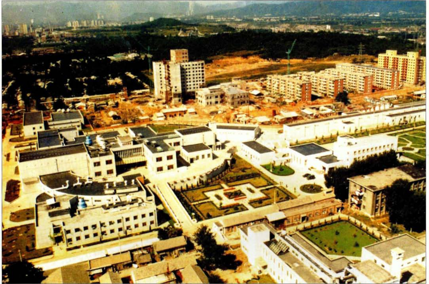
Aerial view of the Beijing Electron-Positron Collider complex at the Chinese Institute of High Energy Physics, showing the buildings that house the circular tunnel of the 240 m circumference collider ring (centre left) and its injector (centre right). The plan is to build a second ring adjacent to the first within the same housing.
