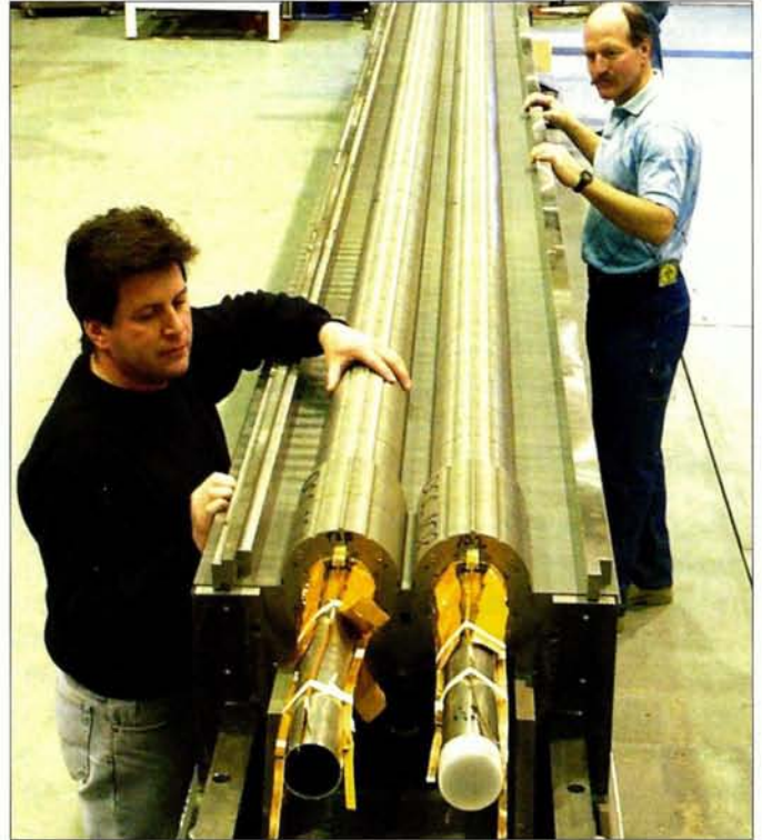
US contribution to the LHC – superconducting separator dipole made by the US Brookhaven Laboratory.
