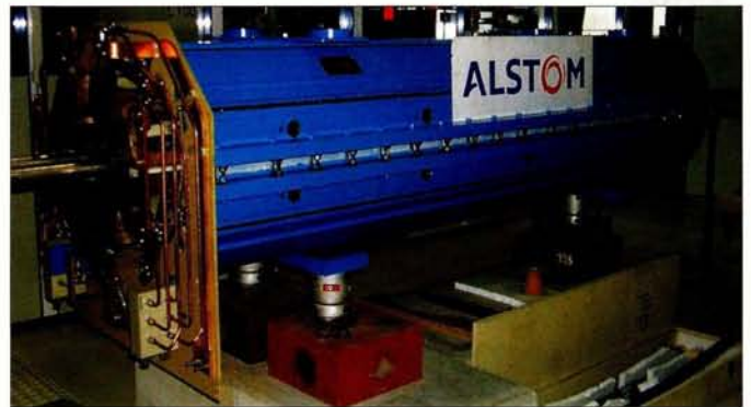
Canada: the first series production twin-aperture quadrupole produced by the TRIUMF laboratory, Vancouver, with ALSTOM Canada.
