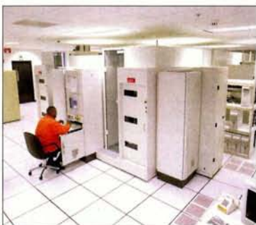
Two "farms" of PCs at Fermilab. Such clusters have largely replaced multiprocessor mainframes.
