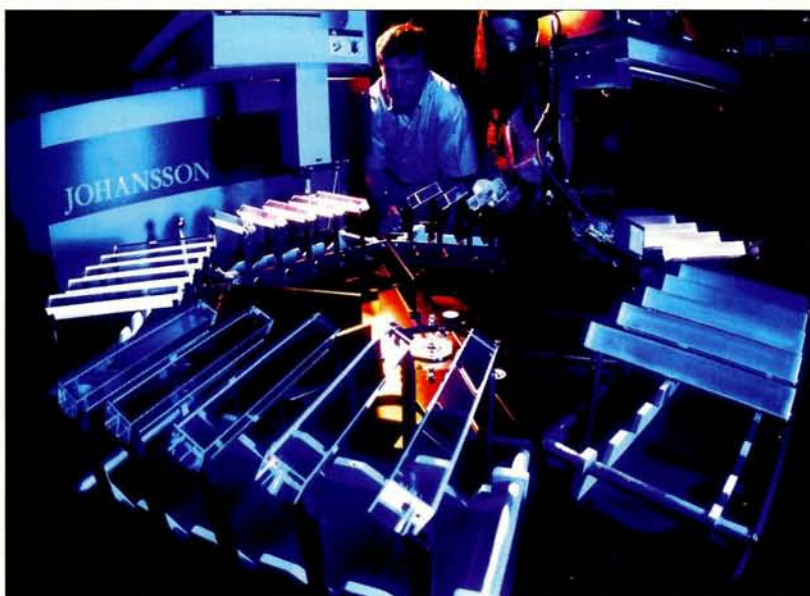
Lead tungstate crystals for the CMS experiment at CERN's LHC. The decision to go for lead tungstate was the result of research and development work by the Crystal Clear collaboration at CERN. The crystals detect the tiny scintillations produced by electromagnetic interactions.
